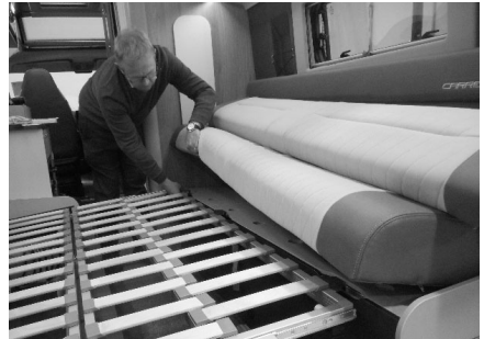
Step 5: Moving to the end of the bed lower the extended bed frame over the off side seat base.
