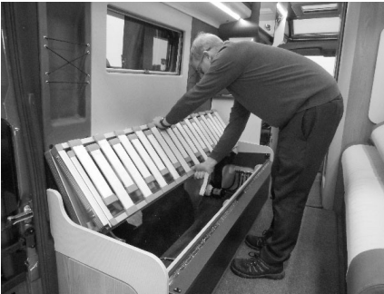
Step 3: Standing in the middle of the bed unfold the seat base..
