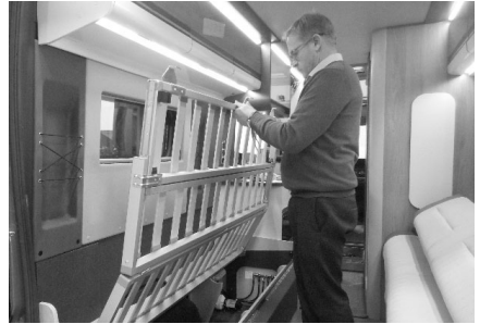
Step 4: Standing in the middle of the bed pull upward the sliding section of the frame..
