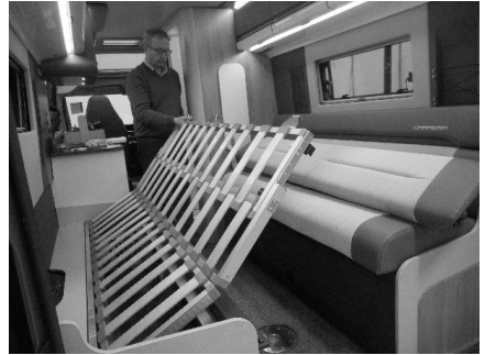
Step 5: Moving to the end of the bed lower the extended bed frame over the off side seat base.
