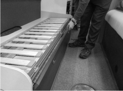
Step 1: Remove the Near side bed cushions and release the front fascia flap at the top of the bed
