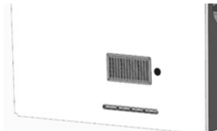
Typical fan switch position, on end of forward furniture near entrance door
