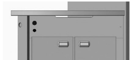
Typical 2nd thermostat and switch installation
