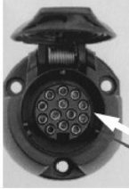
Fig. 3 - Socket body (containing female socket terminals) fitted to the car
