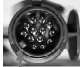
Incorrect alignment Fig. 6
